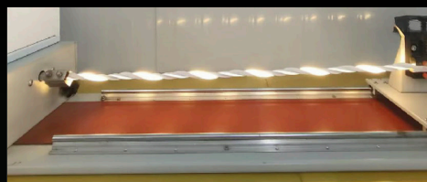
Twist Test 200 times rotating, 360°
