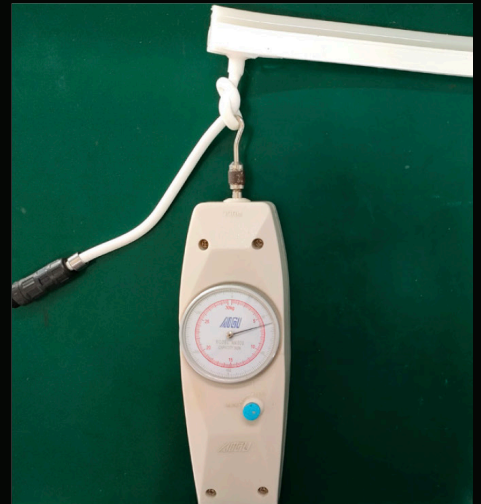
End Cap Tensile Test Four times neon weight
