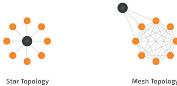
Star topology vs mesh topology
