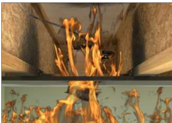
RECESSED LIGHT IN UNPROTECTED CEILING OPENING
