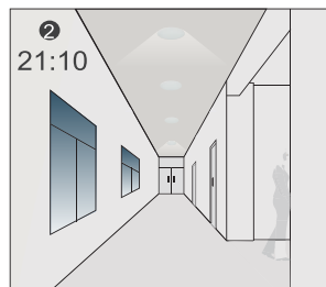
The light dims to stand-by level after the hold-time.
