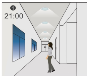
The light switches on at 100% when there is movement detected.
